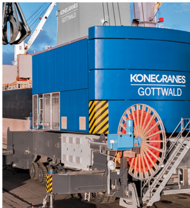
External power from the terminal's electricity supply increases the efficiency of the drive and eliminates local exhaust and noise emissions from the terminal. Surplus energy can be fed back into the on-shore grid.
