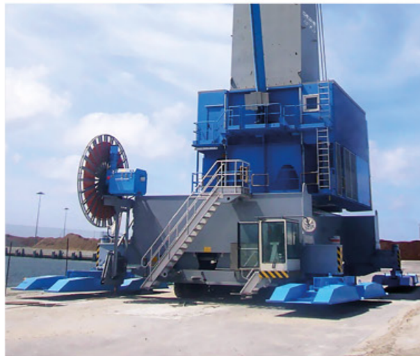
External power from the terminal's electricity supply increases the efficiency of the drive and eliminates local exhaust and noise emissions from the terminal. Surplus energy can be fed back into the on-shore grid.
