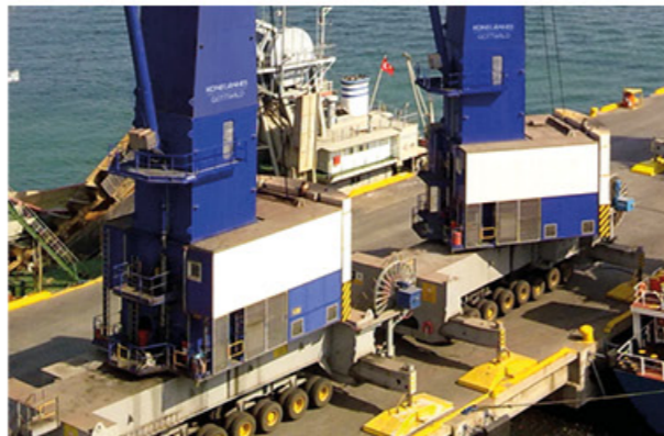
We adapt your mobile harbor cranes to new cargo-handling requirements. For instance, we increased the height of the towers on existing cranes so that vessels with more container layers can be loaded or unloaded on deck.
