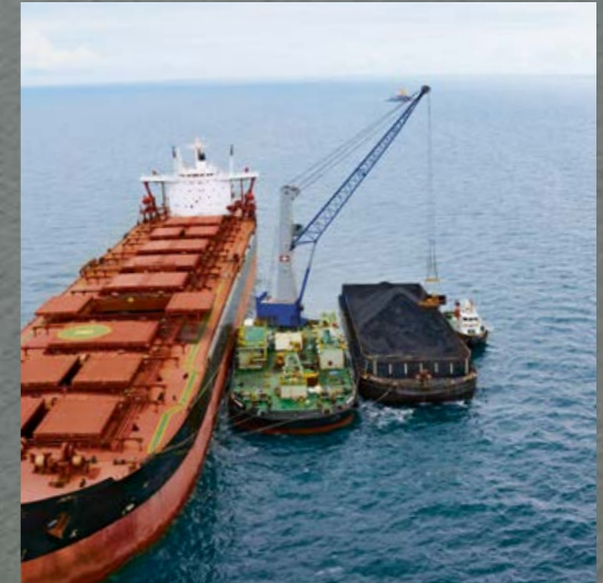
For limited and missing quay infrastructures Konecranes offers floating cranes.
