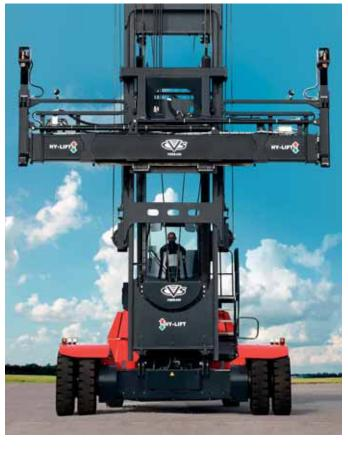
HY-LIFT features a extra wide front axle with a best in class front track that, along its wide steer axle and extended wheelbase, deliver the best LATERAL STABILITY ever featured by a dedicated empty container handler. A unique and first ever lateral stability electronic control system automatically reduces drive speed based on actual stability reserve.
