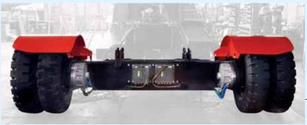
Drive is also electric motor operated. Motors are directly mounted at the wheels and are the same of those operating the winches. Inverters - one per each motor - provide responsive control and exceptional and progressive acceleration. The electric brake is supplemented by a wet disc brake system.
