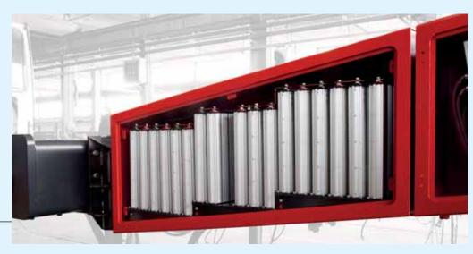
A second source of power is delivered to HY-LIFT by a rack of supercapacitors. Charged by the generator or by recovered energy captured when lowering and braking, the supercapacitor integrate the energy provided by the generator boosting the performances of the machine to levels equivalent to or superior to those of conventionally powered trucks. The supercapacitors come with a manufacturer design life of one million cycles.
