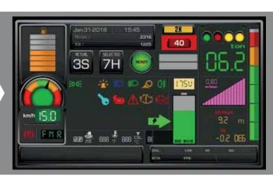
HY-LIFT also features a longitudinal stability LMI. Drive speed, tilt and lift are limited according to residual stability reserve, to lift safety to levels never reached before
