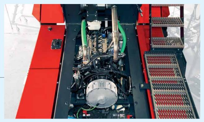
The primary power source of HY-LIFT is a small electric generator actioned by a 90 kW engine. This power pack delivers excellent durability due to regulated engine revolving regime plus low fuel consumption, reduced noise and lower emissions. Then factor in inexpensive maintenance and drastically reduced engine overhauling and replacement cost.
