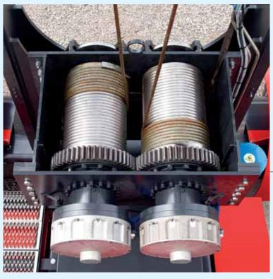
Lifting is achieved through electric motor driven winches reeling steel ropes. No power hydraulics are involved. HY-LIFT delivers maximum efficiency in energy use and recovery, high lifting speeds, total safety granted by three independent brake systems, along with drastically reduced maintenance costs. Total reliability.
