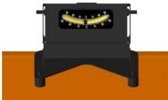
The inclinometer (positioned on the top of the feed funnel) indicates the angle of incline of the chipper, on the horizontal plane. The chipper can operate continuously at a 20° incline and up to 10 minutes at 30° incline.
