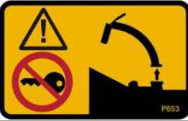
P653         | Danger.<br>Rotating blades inside.<br>Stop engine and remove key before removing discharge unit.                                                       |
