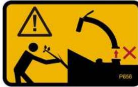
P656         | Danger.<br>Do not use this machine without the discharge unit fitted. Failure to comply may result in serious injury or damage.                        |
