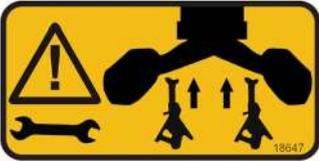
18647      | Appropriate supports must be used while servicing the jacking legs.                                                            |
