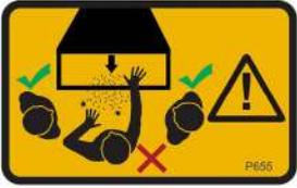
P655         | Caution.<br>Avoid standing directly in front of feed funnel to reduce exposure to noise, dust and risk from ejected particles. |
