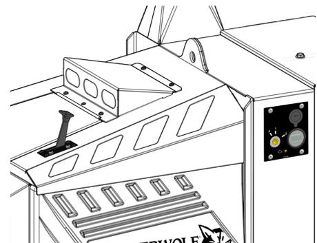
Figure 7 - Throttle Lever and Control Panel
