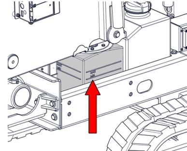
Figure 21 - Hydraulic Oil Level Indicator
