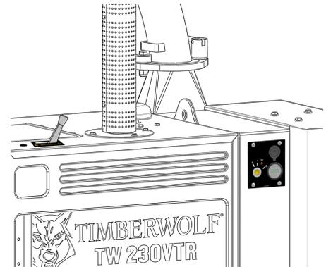
Figure 7 - Throttle Lever and Control Panel
