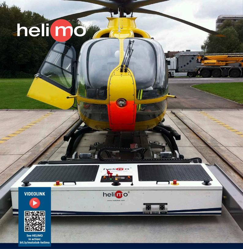
Helimo – the electrical and precise mover for all helicopters with landing skids.
