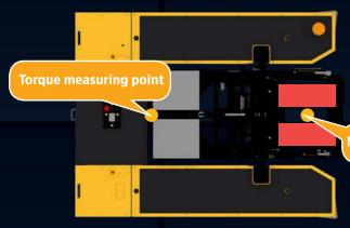
The forces and torques acting on the nose gear are measured by several weighing cells. Mototok's Intelligent Nosegear Protection System (i-NPS) prevents too high torques and initiates a counter steer action whilst either pulling or pushing the aircraft.
