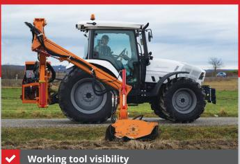
Specially designed crane arm kinematics bring the working tool in the user's visual field, increasing the mowing visibility and the safety of operation.
