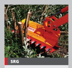
SRG are branch cutters, specially designed for removing the tops of trees as well as large and small vegetation up to 100 mm thick.
