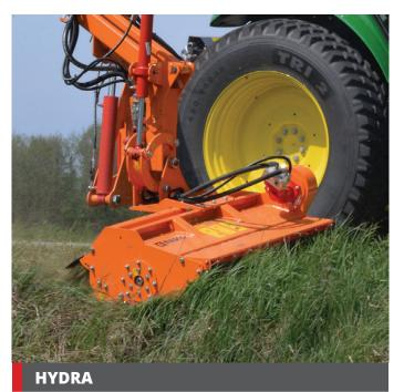
HYDRA is a combined operating head for mowing and fragmenting vegetation up to 50 mm thick. Efficient operation of the HYDRA mowing head is enabled by the design of its key parts. The spiral distribution of blades reduces energy loss, and an increased aperture on the rear end of the head enables high outflow of material, and accordingly, a higher mowing speed.
