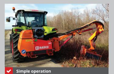
SPECTRA rear crane mower is simple to mount and demount from the rear three-point attachment, quickly equipping the tractor for the mowing season as well as quickly freeing it for other purposes.
