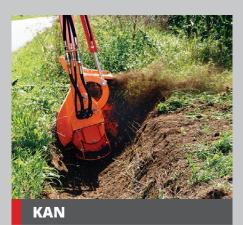
KAN is a ditch cleaner, designed for cleaning and profiling ditches by the side of roads.
