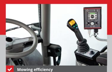
Advanced intuitive control system enables simple operation of the crane arms and the working tool, while the external oil cooler next to the aggregate prevents overheating of the oil, ensuring long-lasting and uninterrupted mowing.
