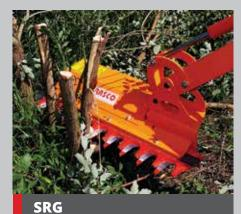
SRG are branch cutters designed for removing the tops of trees, as well as large and small vegetation up to 100 mm thick.
