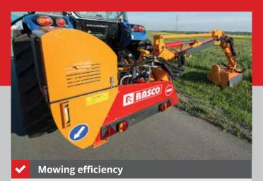
The advanced intuitive control system ensures easy operation of the crane arms and working tools, while the external oil cooler located next to the hydraulic power unit prevents the oil from overheating and ensures long-lasting and uninterrupted mowing.
