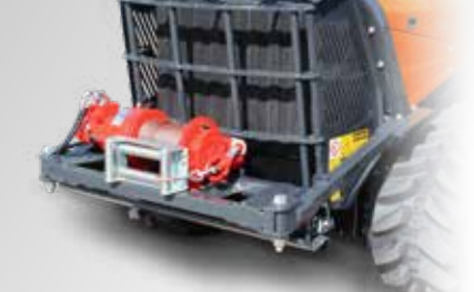
WINCH VERRICELLO POSTERIORE REAR WINCH
