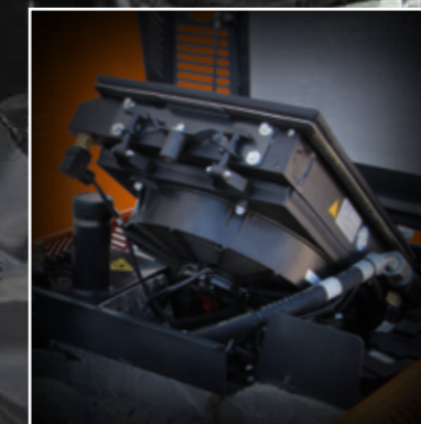
VENTOLA AUTOPULENTE IDRAULICA HYDRAULIC SELF-CLEANING FAN
