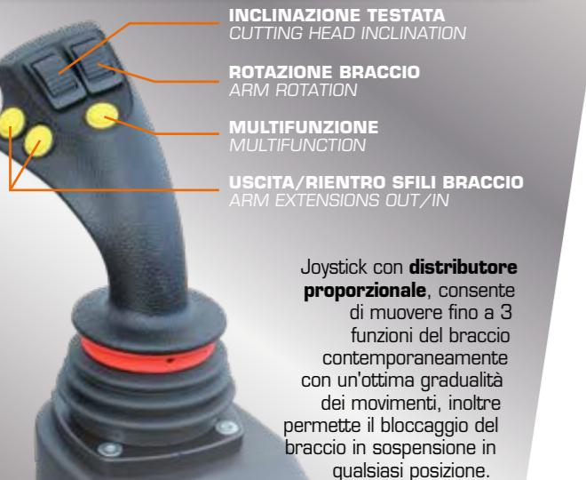
Joystick equipped with a **proportional distributor**, it allows you to move up to 3 arm functions at the same time with an excellent gradual movement, and also allows the arm to be suspended in any position.
