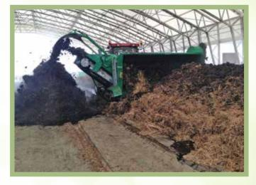
The TracTurn combines the loosening, aerating, mixing and side stacking of the material in one step to the right side (on demand also to the left side). Durability and capacity together with its flexibility to be working in any sort of pile shape, its short setup-time from transport to working mode (only 10 min) make it possible to serve several sites with one machine and can additionally boost the economy of the machine and the tractor.
