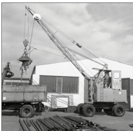
1962: rope-driven S833 with elevated operator cab
